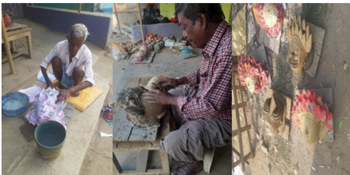
These pictures show different stages of the Chhau mask-making process: paper layering, applying clay and keeping for sun drying (left to right).
